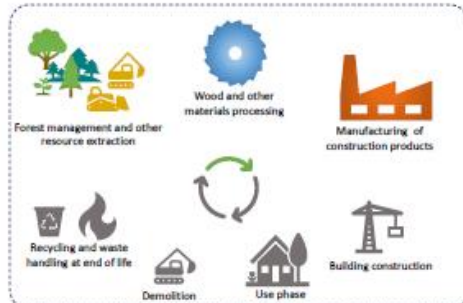
Figure 1: System boundary for the LCA. Transport is also included but not shown in the figure. Only the coloured life cycle stages are reported in this first iteration.
