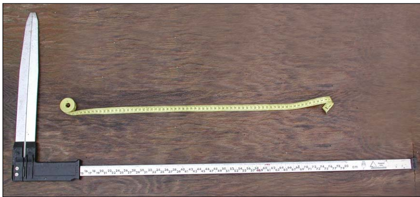
Fig. 66. Tools used to measure the animal: a nonstretching tape measure and large sliding calipers (tree calipers).
